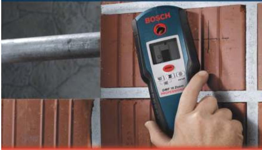
Wherever drilling is required, inductive detection provides additional safety for the operator. The DMF 10 Zoom with the unique "Zoom" function accurately detects metal objects, wooden substructures, live and non-live power cables hidden in masonry, thus putting an end to expensive drilling damage and enabling safer drilling. The detector provides intuitive operation and includes added features like the high-resolution 5-segment display panel, LED ring and the integrated marker pen.
